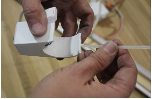
Stuff the ends of the wires into the switch pod as shown.
