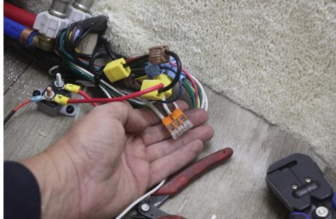
If you have a fuse link like in the picture, simply connect the ring terminal of the power module to one post of the fuse link.
